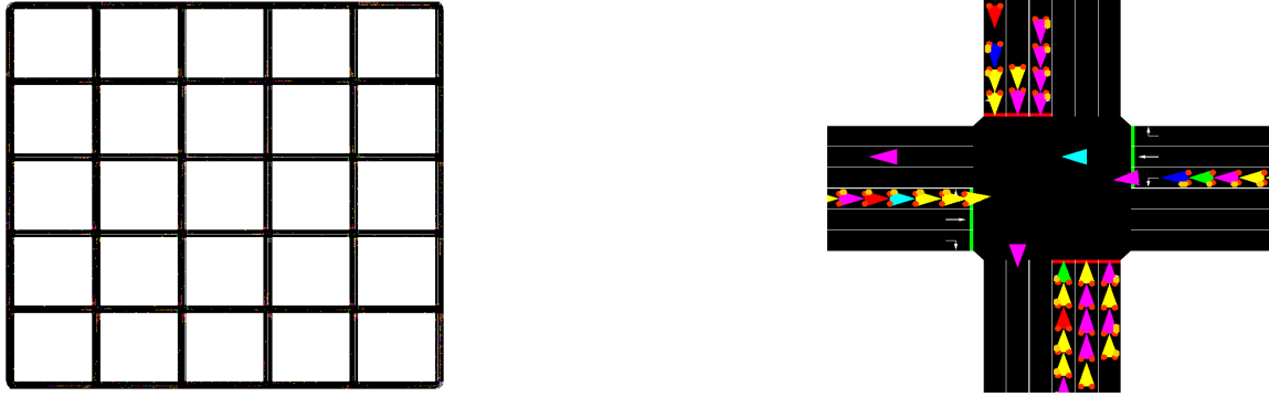
Figure 3.5: (Left) The city layout in the simulation. It is an 1km x 1km area (each segment is 200 meters). (Right) The detail of an intersection in the city layout. Each intersection has traffic lights enabled, the vehicles (here the triangle-like icons stand for vehicles) pile up there.
