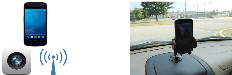
Figure 2.2: (Left) Smartphone has camera and wireless component. (Right) It is mounted on dashboard or windshield in vehicle when using OmniView.
